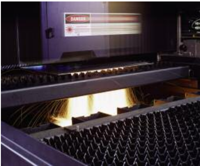
Gortite® Way Protectors on a beam path for a high-tech laser-cutting machine.
