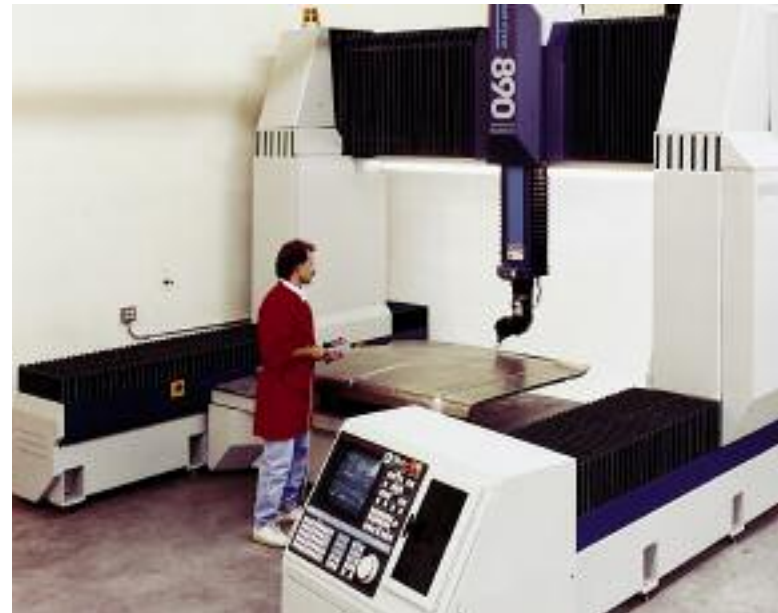
Heat-sealed crossrail and bedway covers keep contaminants from damaging linear rails on a laser cutting machine.
