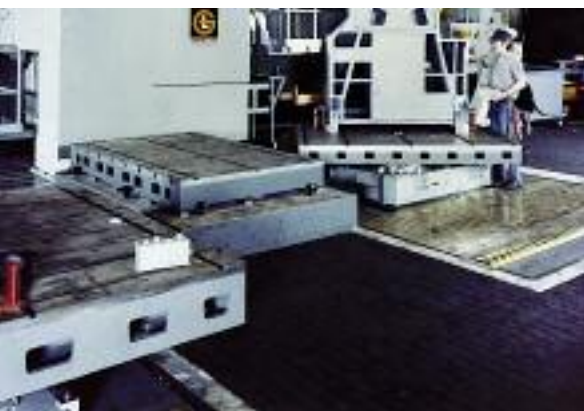
Steelflex® protects machine ways from damage while covering pit opening for operator safety and machine accessibility.
