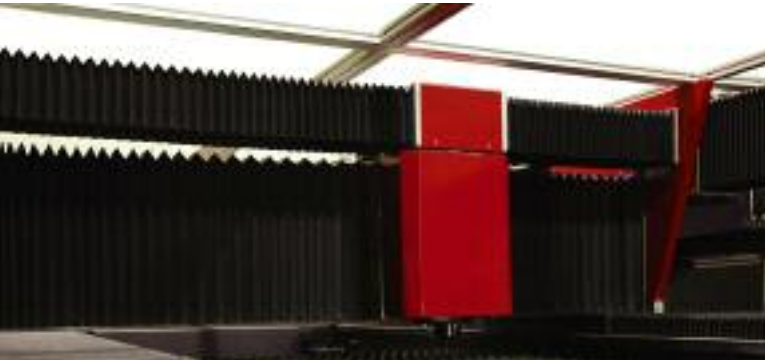
Enclosed Rectangular Beam Path Bellows plus a Way Protector gantry bellows on a laser cutting machine.
